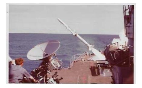
From editor's files: Terrier missile fired from aft launcher of USS Reeves (CG-24).
